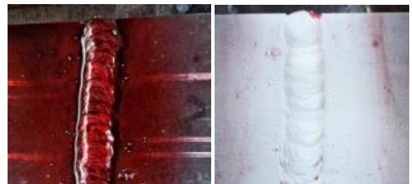
Gambar 6. Hasil Penetrant Test
