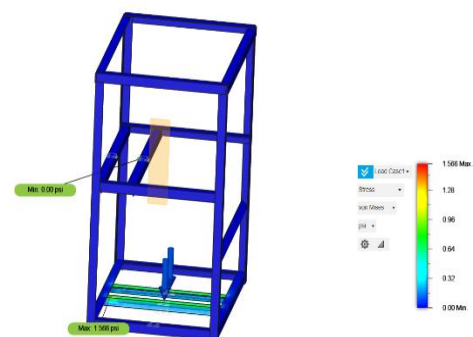
Figure 9. Maximum Stress Results from FEM Simulation
