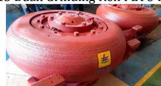
Gambar 1 Grinding Tyre Pulverizer Coal Mill
