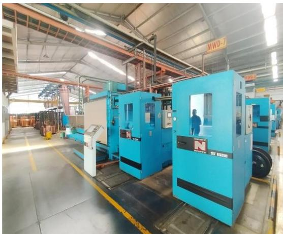
Gambar 2. Mesin *multi wire drawing*
