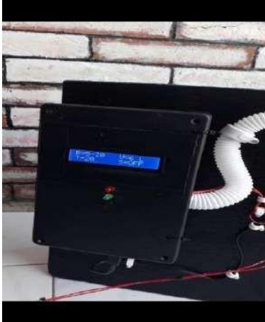
Figure 12. Display of Water Level Information
