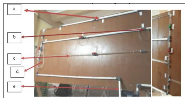
Gambar 3. Proses assembly alat peraga pompa paralel
